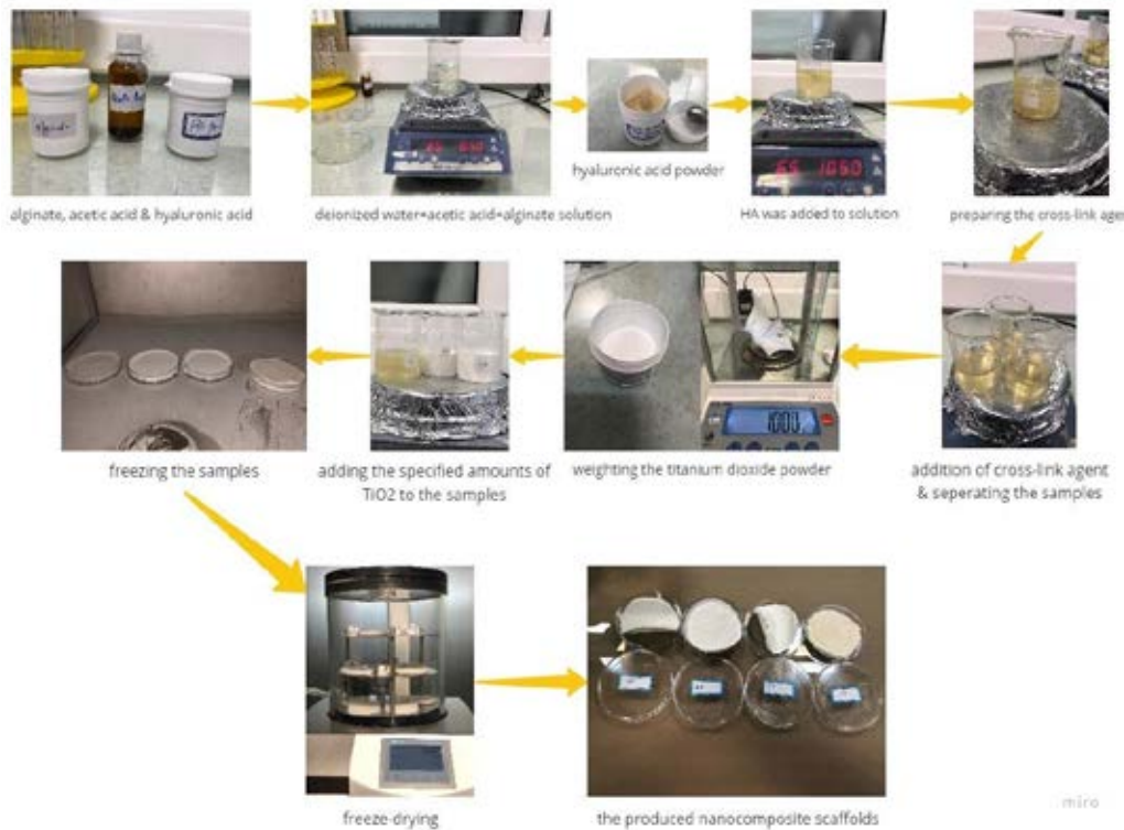
Fig. 1: Schematic of alginate-hyaluronic acid nanocomposite containing titanium oxide nanoparticles.
