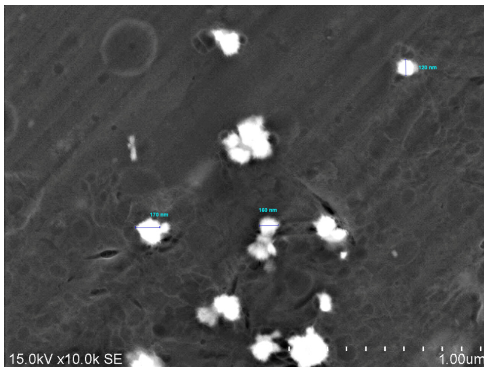
Fig. 3. Scanning electron micrograph of CA-MOX nanoparticles to support the morphology.
