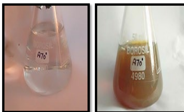
Figure 1. Colour changes in the P. emblica leaves extract after addition of silver nitrate (1 mM aqueous solution of AgNO 3 ) for nanoparticles synthesis
