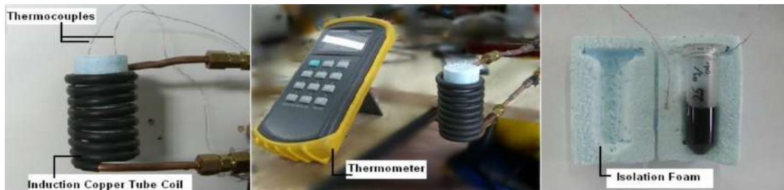
Fig 2. Experimental setup where MNPs in different concentrations were placed in an isolation foam that was fitted for the inside of the cylindrical coil attached to the hyperthermia machine. Thermocouple probes measured the temperature of the MNPs and the isolation foam.
