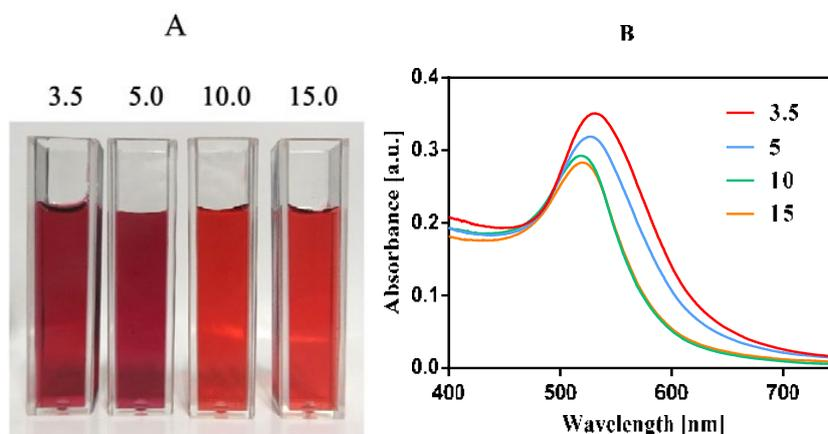
Fig.1. Image (A) and UV-vis spectra (B) of gold nanoparticles samples that synthesized via 'inversed Turkevich' method at various Sodium citrate/HAuCl<sub>4</sub> molar ratios: 3.5, 5.0, 10.0, and 15.0.
