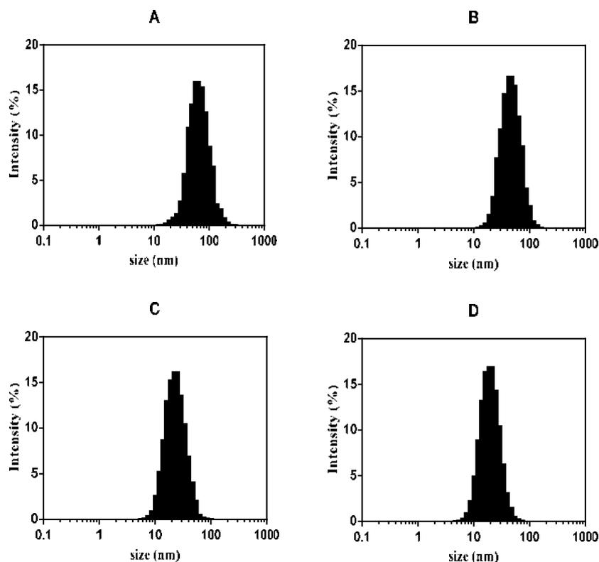
Fig. 2. Size distribution based on light scattering intensity (%) of gold nanoparticles samples that synthesized at different Sodium citrate/ $\text{HAuCl}_4$  molar ratios: A) 3.5, B) 5.0, C) 10.0 and D) 15.0.
