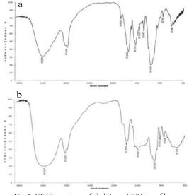
Fig. 5. FT-IR spectrum of;a) chitosan/PEO nanofibers b) chitosan/PEO/cefazolin nanofibers
