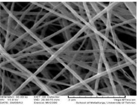
Fig. 1. SEM image of chitosan/PEO nanofibers with ratio of 90 to 10
