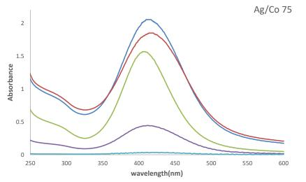
Fig. 4: Absorption spectra of silver-cobalt nanoparticles produced from silver nanoparticles at a different time interval of 75 seconds on the first, second, third, seventh, and fourteenth days (The electrical current adjusted at 1 amp and rotational speed was 3000 rpm).
