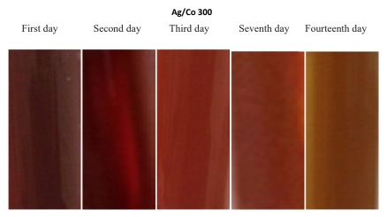
Fig. 5: Silver-cobalt nanoparticles produced from silver nanoparticles at intervals of 300 seconds on the first, second, third, seventh, and fourteenth days (respectively, from left to right)
