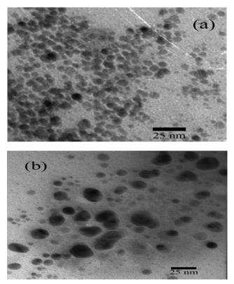
Fig. 7: TEM image of silver-cobalt nanoparticles produced (a) of silver nanoparticles synthesized during 75 seconds, (b) of silver nanoparticles synthesized in a period of 300 seconds (The electrical current adjusted at 1 amp and rotational speed was 3000 rpm).
