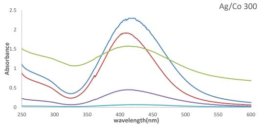
Fig. 6: Absorption spectra of silver-cobalt nanoparticles produced from silver nanoparticles at a different time interval of 300 seconds on the first, second, third, seventh, and fourteenth days (The electrical current adjusted at 1amp and rotational speed was 3000 rpm).
