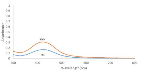
Fig. 2: Absorption spectra of silver-cobalt nanoparticles prepared from silver nanoparticles synthesized at intervals of 75 seconds and 300 seconds (The electrical current adjusted at 1amp and rotational speed was 3000 rpm).
