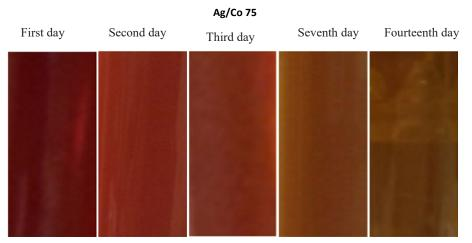
Fig. 3: Silver-cobalt nanoparticles produced from silver nanoparticles at different times of 75 seconds on the first, second, third, seventh and fourteenth days (respectively, from left to right).
